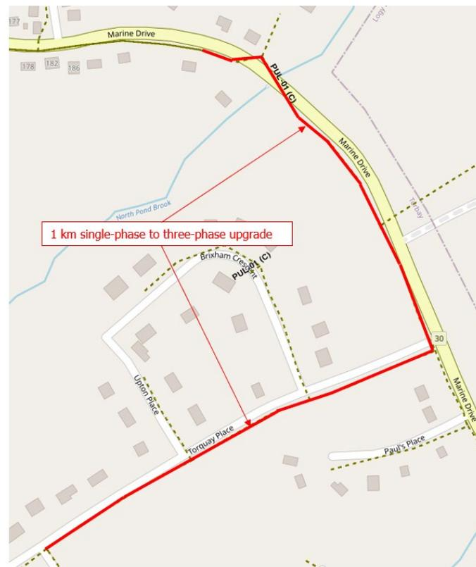
Figure 3: Alternative 2 - PUL-01 Upgrades Along Marine Drive and Torquay Place
