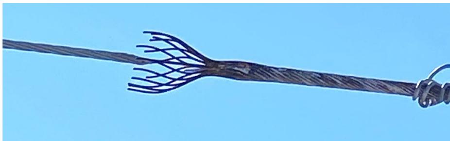
*Figure 3: 2/0 ACSR Conductor Deterioration*
