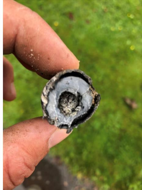
Figure 3: Loop 34 Primary Conductor Failure
