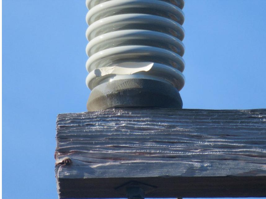
Figure B-3: Cracked Porcelain Insulator
